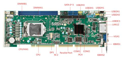
Figure 1: Board Layout: Jumper and Connector Locations
