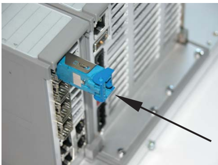
Figure 11: Installing an SFP module
