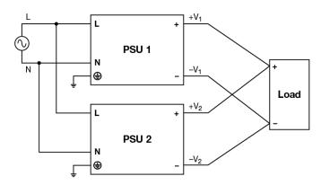
Fig. 4 Parallel Operation Connection Diagram
