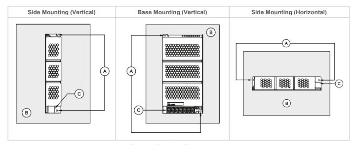
Fig. 2 Mounting Orientation
