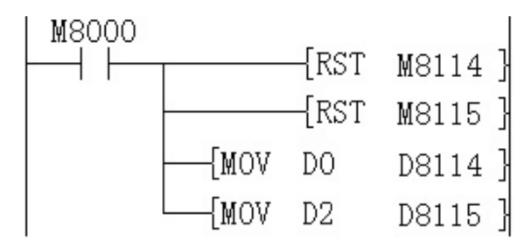
• If the data are not stored into D0 or D2, then D8112, D8113 and D8114, D8115 can be simultaneously used on setting values and other orders, such as timer/counter.
