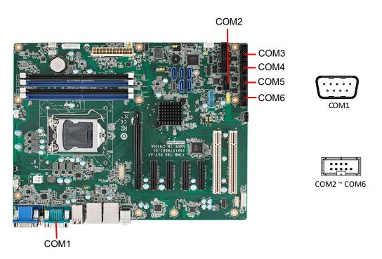
The AIMB-786 offers six serial ports (one on the rear panel and five on-board). COM3 can be configured as RS-232/422/485 by jumper settings (see Chapter 1), and selecting correct device mode for RS-485 under BIOS is necessary (see Chapter 3). These ports can connect to a serial mouse, printer or communications network. The IRQ and address ranges for those ports are fixed. However, if you want to disable the port or change these parameters later, you can do this in the system BIOS
