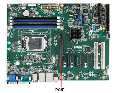
The AIMB-786 provides a PCIe x16 slot for users to install an add-on peripheral card for extension requirements.
