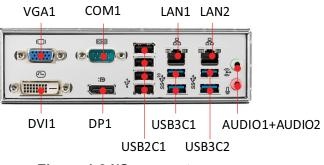
Figure 1.2 I/O connectors
