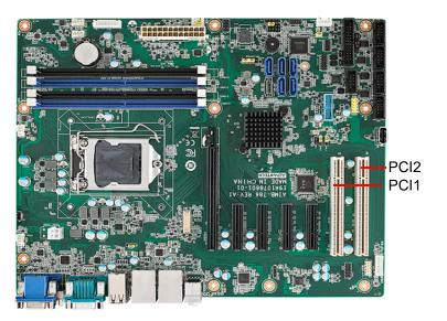
The AIMB-786 provides two 32-bit / 33 MHz PCI slots.
