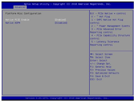
**Figure 3.4 Platform Misc Configuration**
