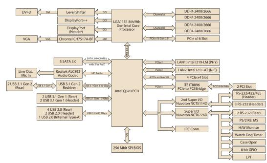
Figure 1.3 Block Diagram
