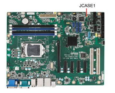
JCASE1 is for chassis with a case open sensor. The buzzer on the motherboard sounds if the case is opened unexpectedly. The default function is disabled and pins 1-2 is bridged by a jumper cap.
