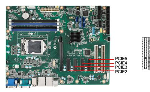
The AIMB-786 offers four PCIe x4 slots for users to install add-on cards for extension requirements.
