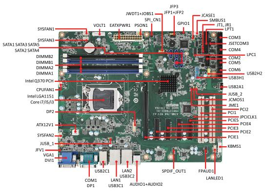
**Figure 1.1 Jumper and Connector Locations**
