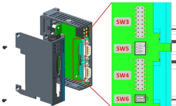
Figure 5.6 AMAX-5490 Jumper Switch
