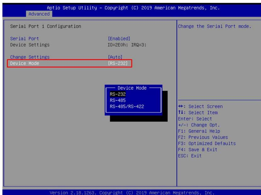
Figure 3.10 Configure serial port protocol type in BIOS
