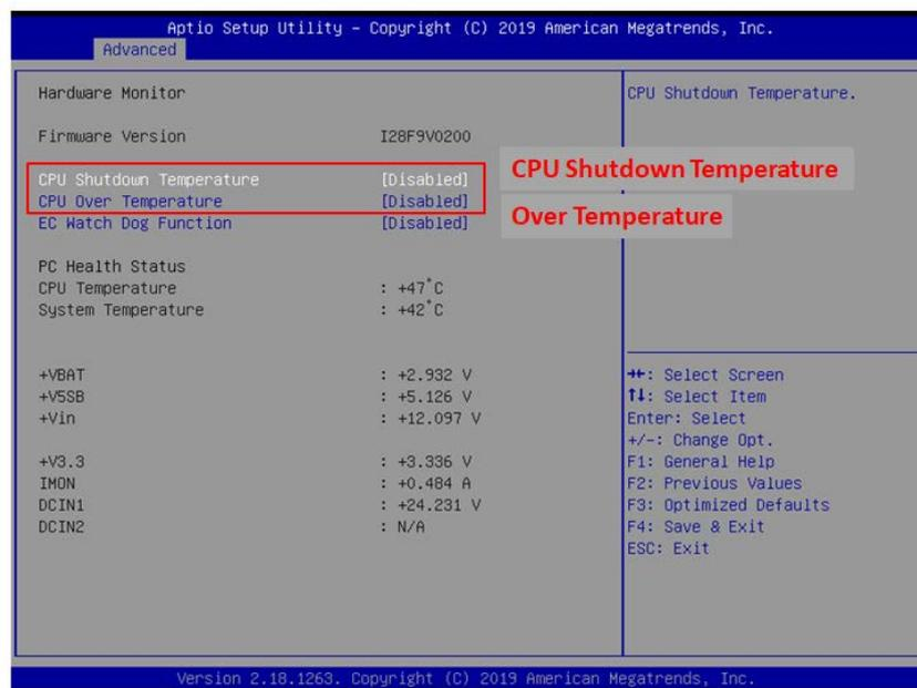
Figure 3.6 The CPU shutdown temperature and overheating temperature configuration in BIOS
