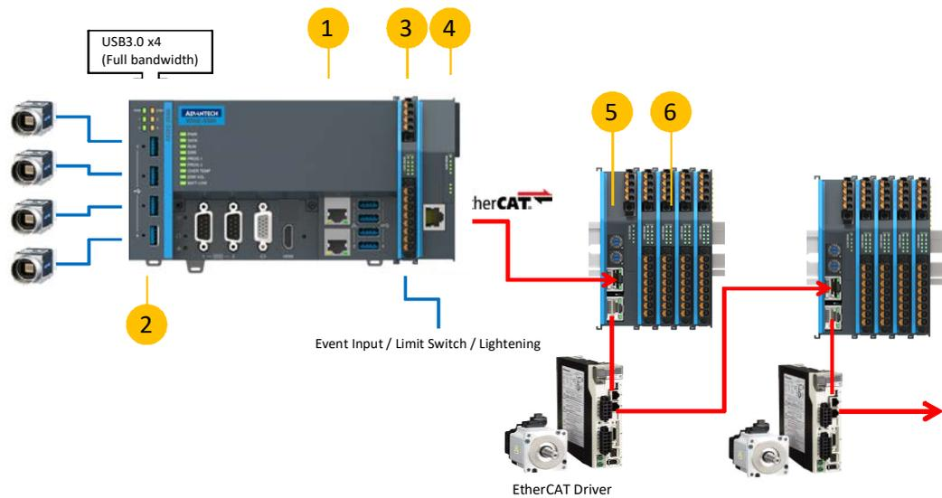
**Figure 2.5 AMAX-5000 System Configuration for Motion + Vision Application**
