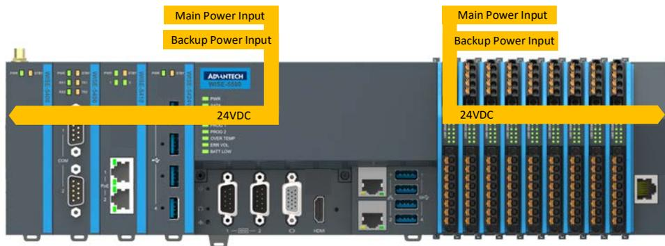
**Figure 2.2 Power System of AMAX-5000**
