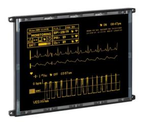
EL640.480-AM LVDS is a VGA-display for use in extreme operating conditions.
