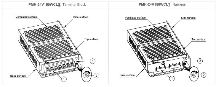
1) Input & Output terminal block connector
