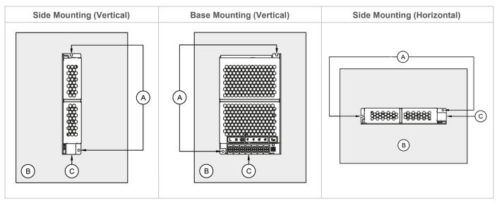
Fig. 2 Mounting Orientation
