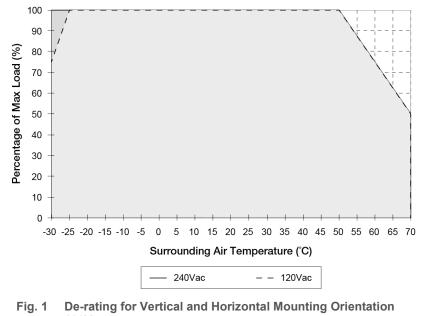
**120Vac** < -25°C de-rate power by 5.0% / °C **120Vac and 240Vac** > 50°C de-rate power by 2.5% / °C
