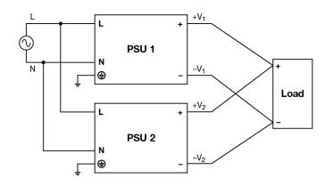
Fig. 4 **Parallel Operation Connection Diagram**
