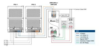
\*\*The Signal GND in the DRR module is for the built-in LED and DC OK signals. The Output GND terminals from the two PSU's do not need to be connected to the Signal GND terminal. Connect the power supply units PSU 1 and PSU 2 to Vin 1
