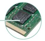
Apacer DRAM module with conformal coating
