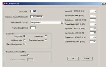
6. Right click onto the master and open the VIPA specific dialog "Set PLC Parameters". Here you may adjust the diagnosis behavior and the address ranges that the master occupies in the CPU. At "Slot number" type the SPEED-Bus slot no. added with 100 (101...110), where your CAN master is plugged. At export, WinCoCT creates the according DB no. + 2000.
