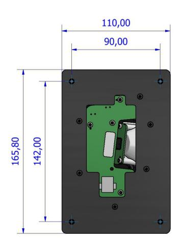
Dimensional drawing specifies factory default orientation. All dimensions are in mm unless otherwise stated. Tolerances +/- 0.25mm unless otherwise stated IGES/STEP model available on request.
