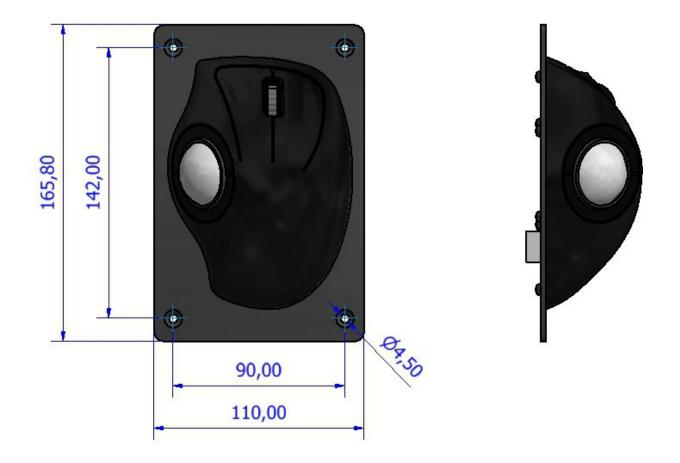
Dimensional drawing specifies factory default orientation. All dimensions are in mm unless otherwise stated. Tolerances +/- 0.25mm unless otherwise stated IGES/STEP model available on request.
