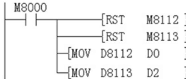
The following program will be set into voltage output mode, and the data of D0 and D2 will be converted into analog value.
