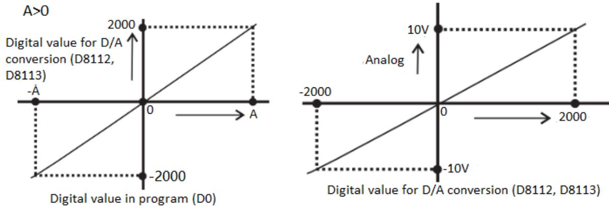
If the figure range used in D0 is -A~A, then the data used in the user's applications are:
