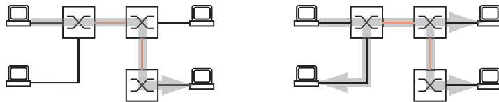
Figure 73: MAC Data Transmission: Unicast Data Packet (left) and Broadcast Data Packet (right)
