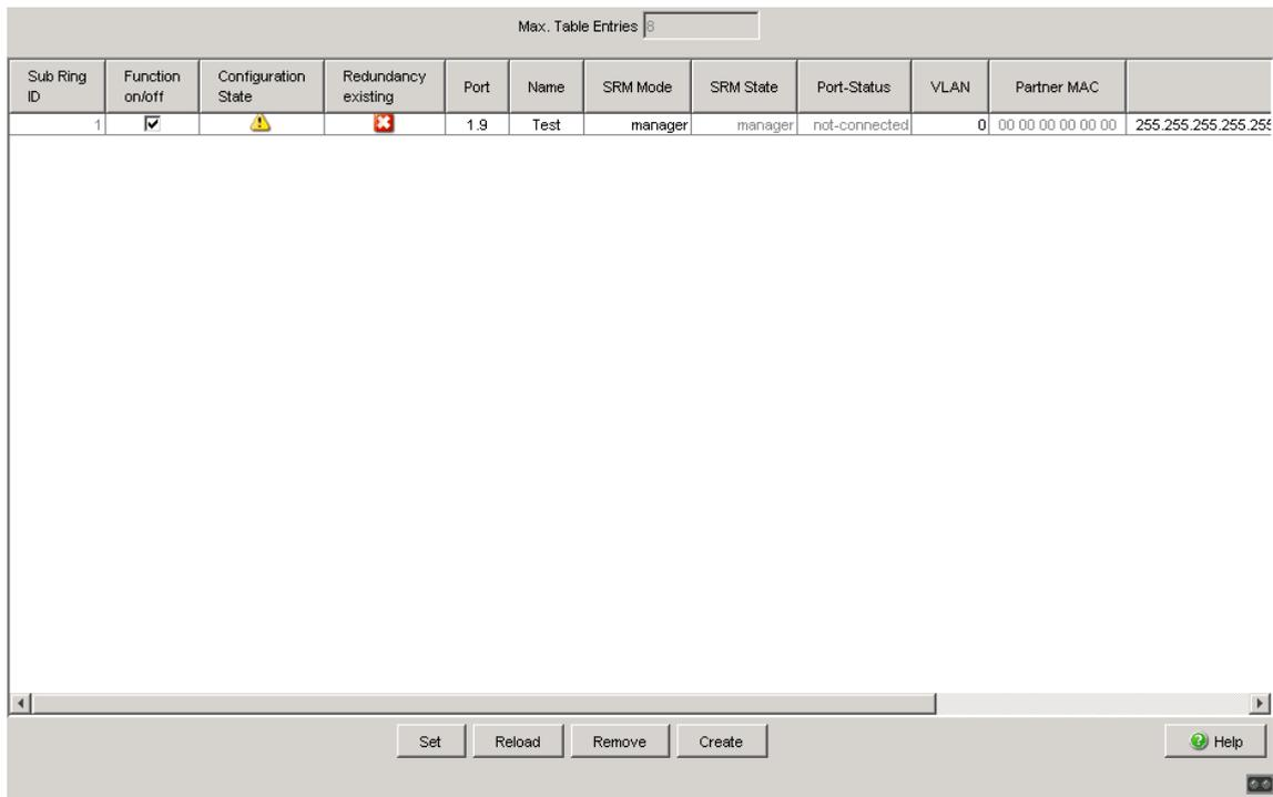
Figure 69: Sub-Ring basic configuration
