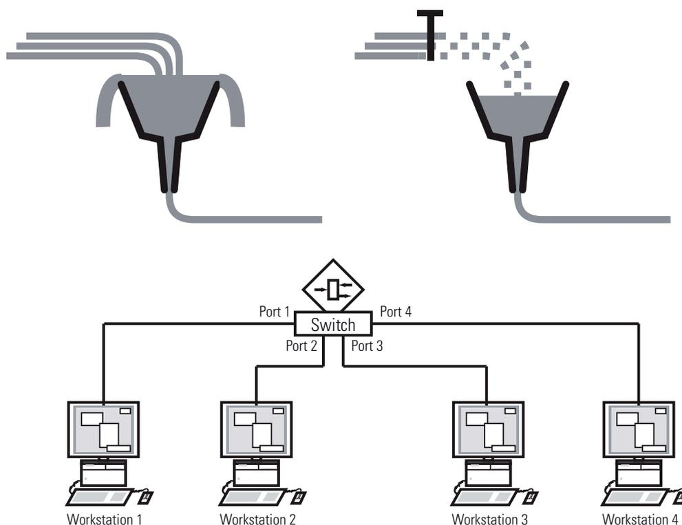
Figure 42: Example of flow control
