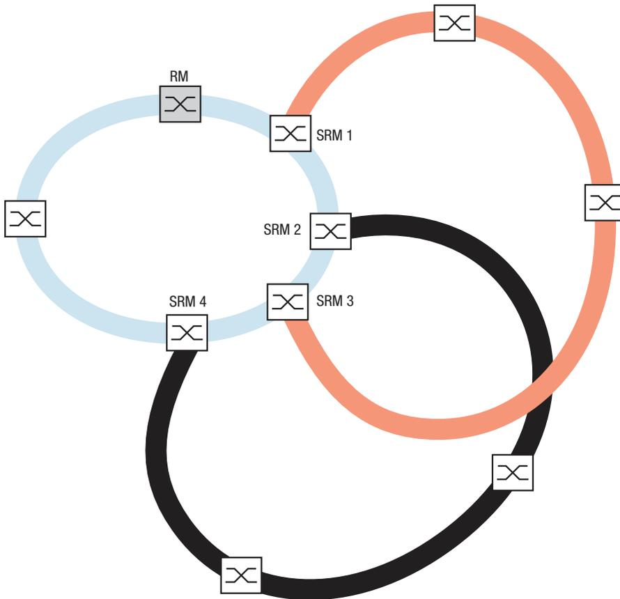
Figure 16: Example of an overlapping Sub-Ring structure
