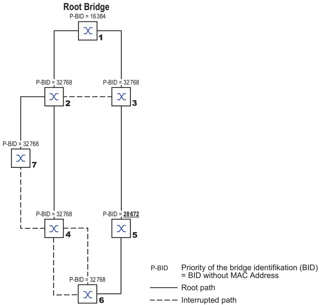
Figure 48: Example of manipulating the root path
