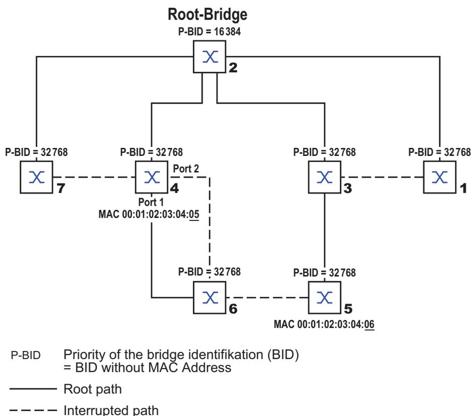
Figure 49: Example of manipulating the tree structure
