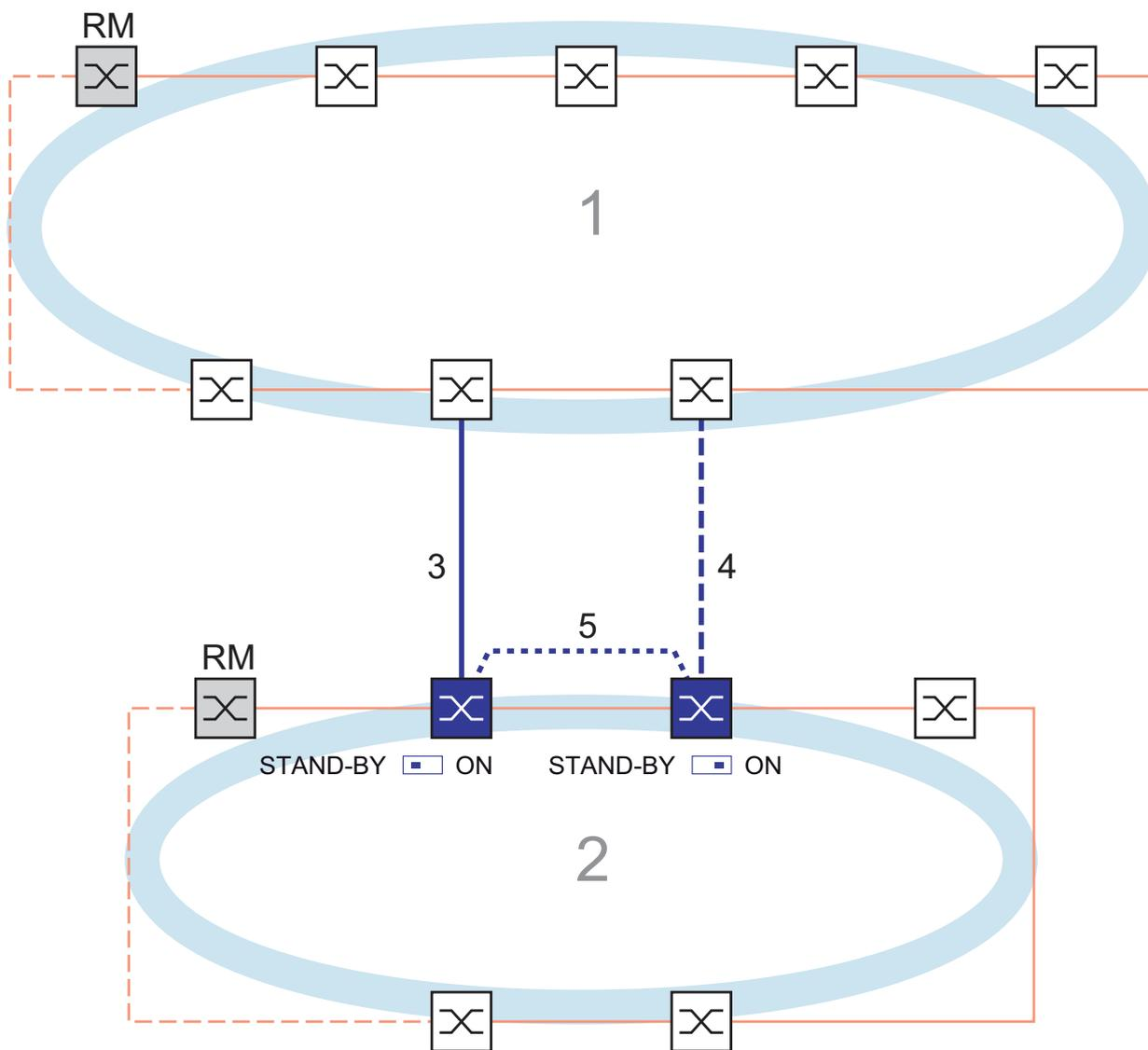
Figure 36: Example of Two-Switch coupling with control line
