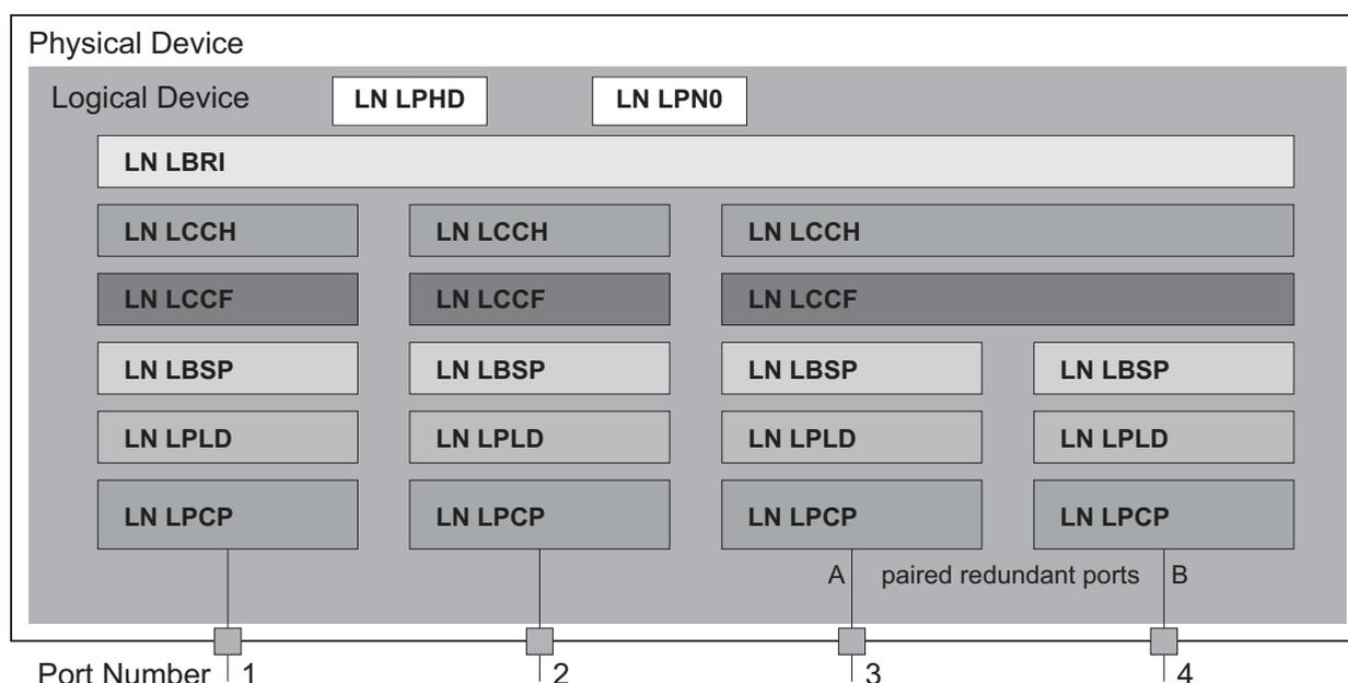
Figure 23: Bridge model based on Technical Report IEC 61850 90-4
