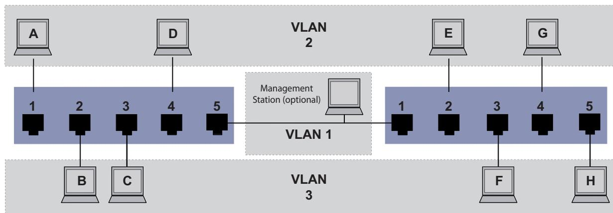
Figure 47: Example of a more complex VLAN configuration
