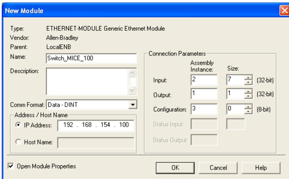
Figure 4: Integrating a new module into Logix 5000
