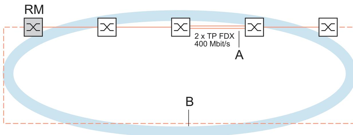
Figure 6: Example of a HIPER-Ring / link aggregation combination
