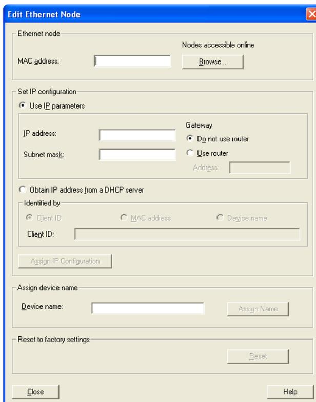
Figure 10: Dialog for entering the Switch name
