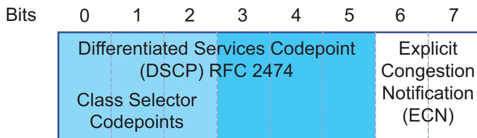
Figure 41: Differentiated Services field in the IP header
