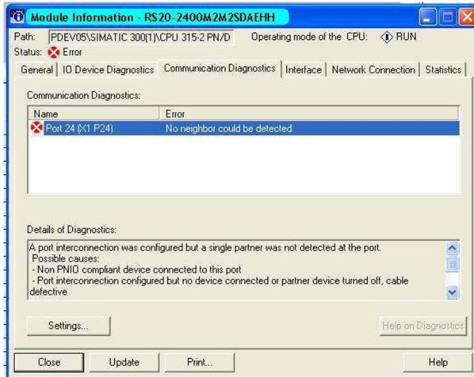
Figure 21: Diagnosis messages for the communication between the Switches and IO devices
