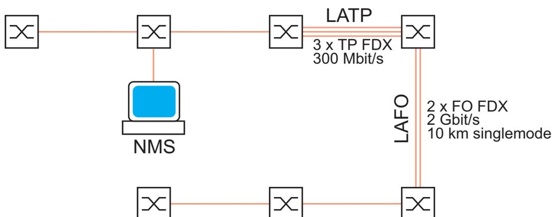
*Figure 1: Example of link aggregation*
