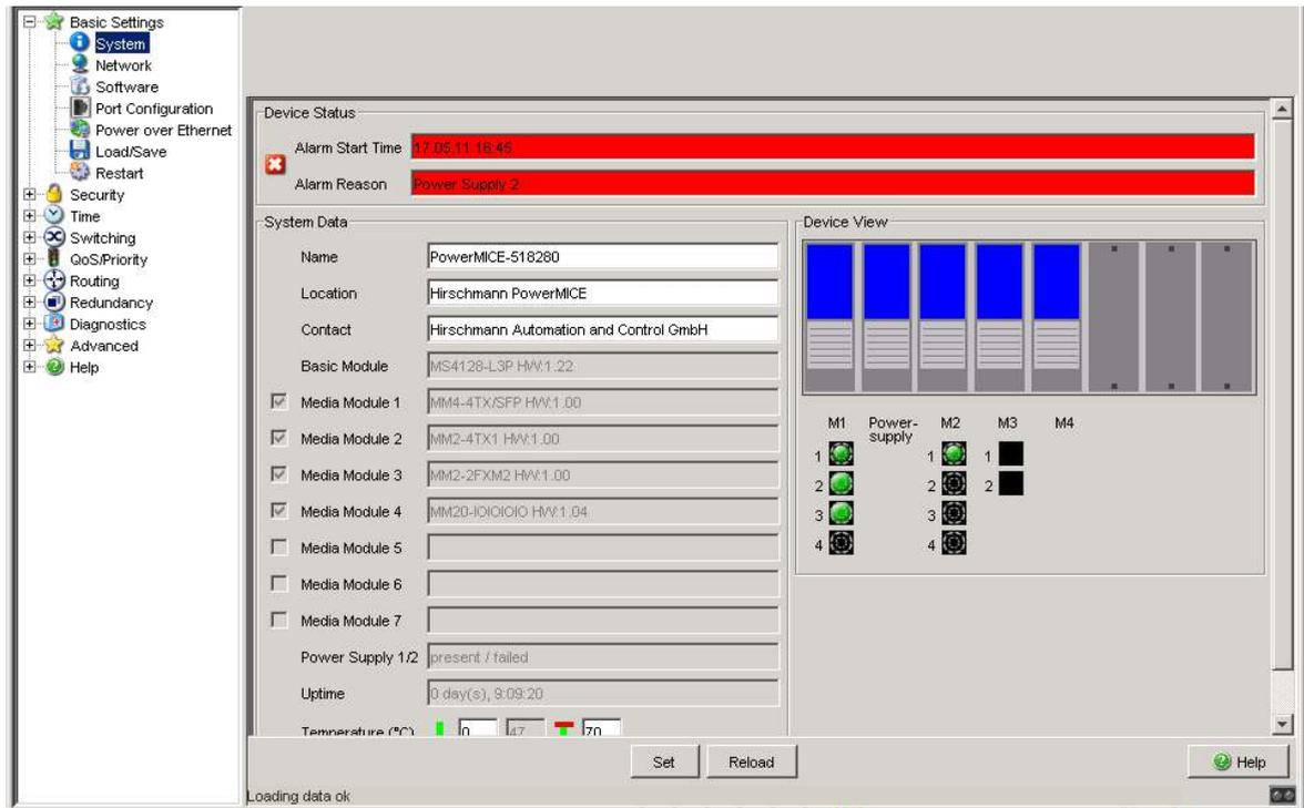
Figure 17: Basic Settings Dialog: System in the Graphical User Interface
