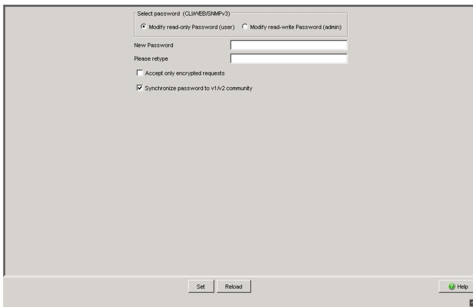
Figure 22: Password/SNMP Access dialog
