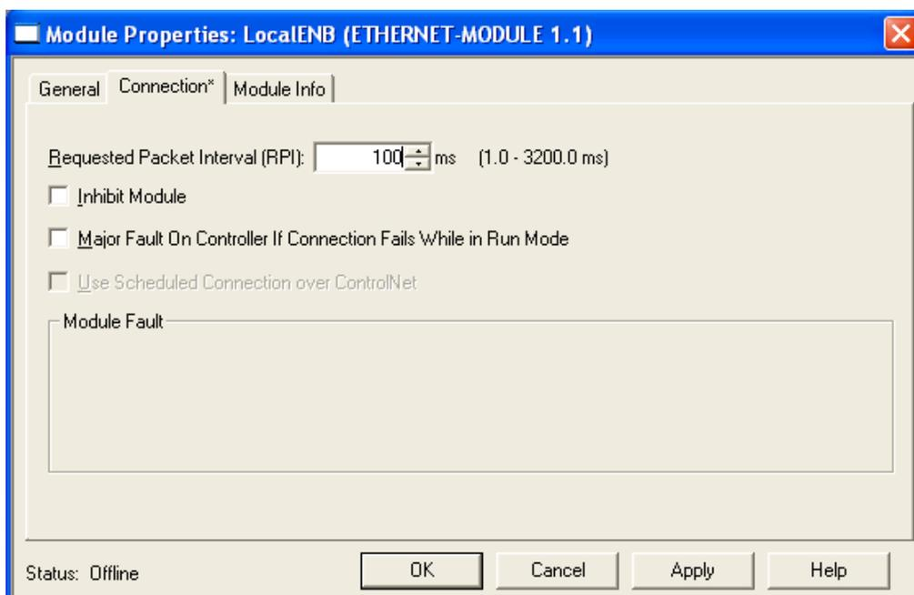
Figure 5: Module properties for the Request Packet Interval (RPI)
