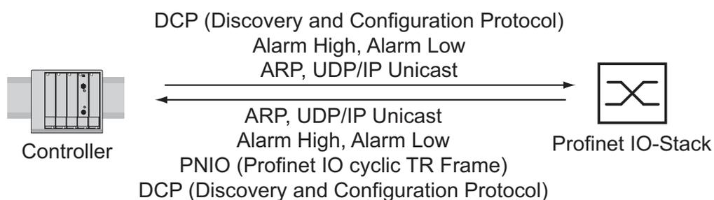
Figure 6: Communication between the Controller and the Switch
