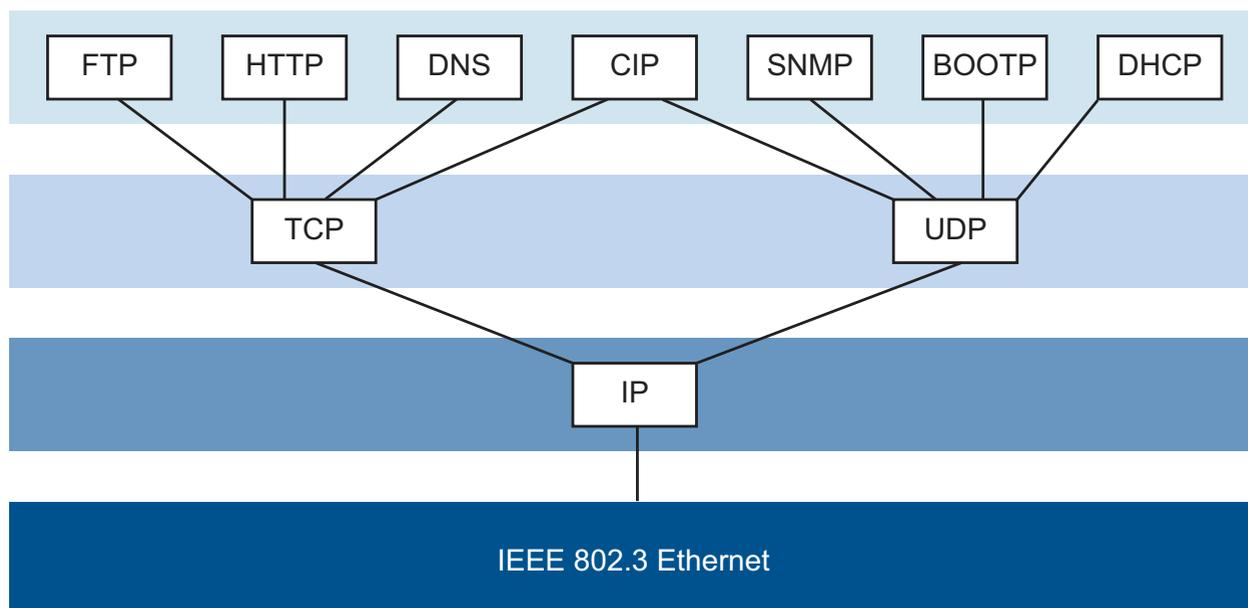
Figure 3: EtherNet/IP (CIP) in the ISO/OSI reference model
