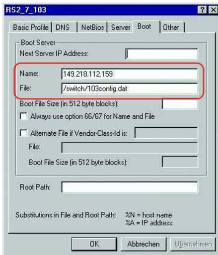
Figure 65: Configuration file on the tftp server
