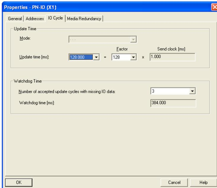
Figure 12: Dialog for entering the IO Cycle
