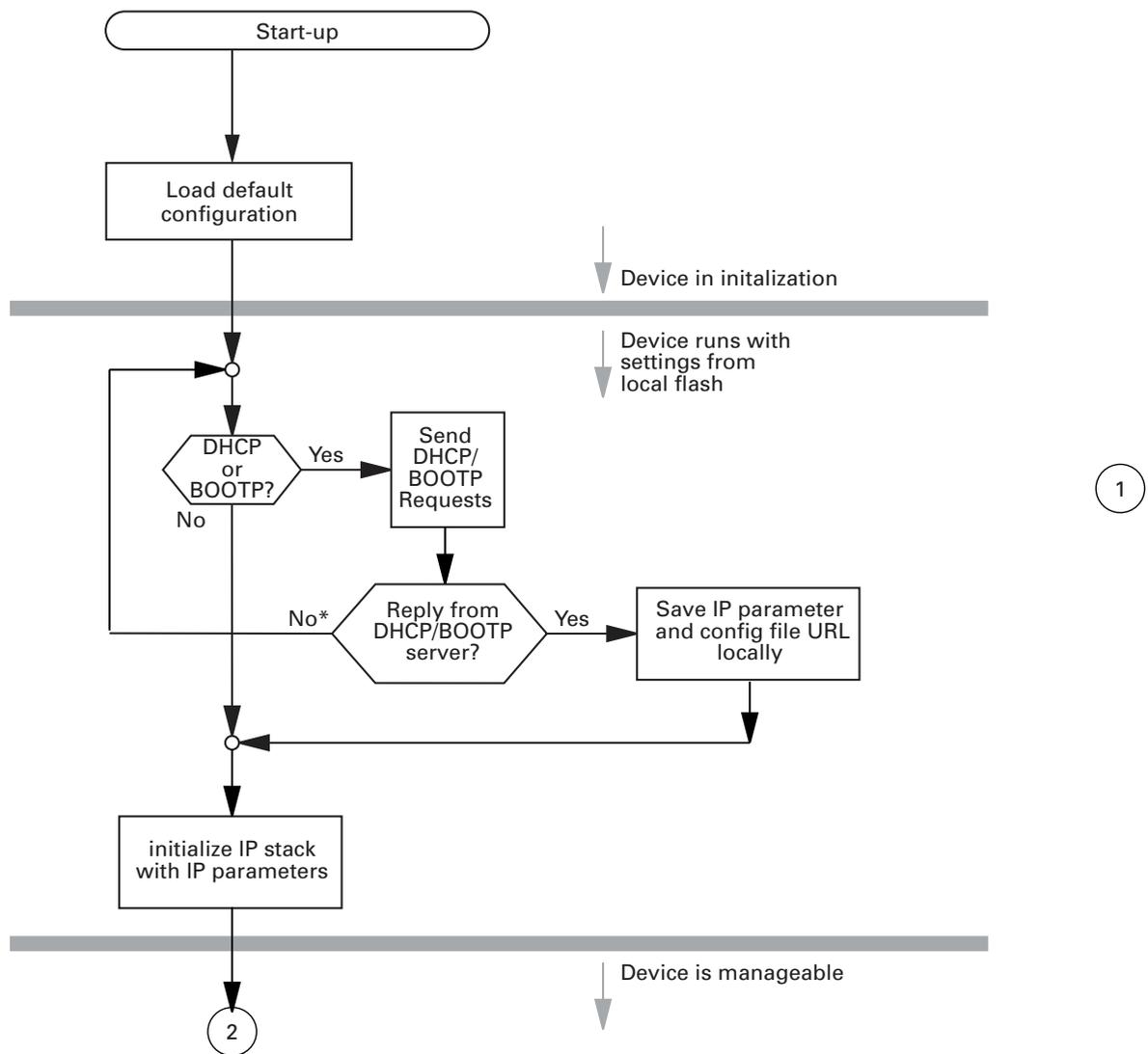
Figure 10: Flow chart for the BOOTP/DHCP process, part 1
