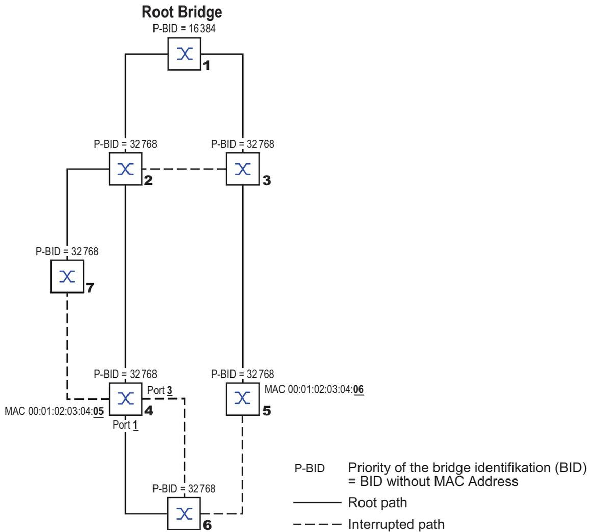
Figure 47: Example of determining the root path
