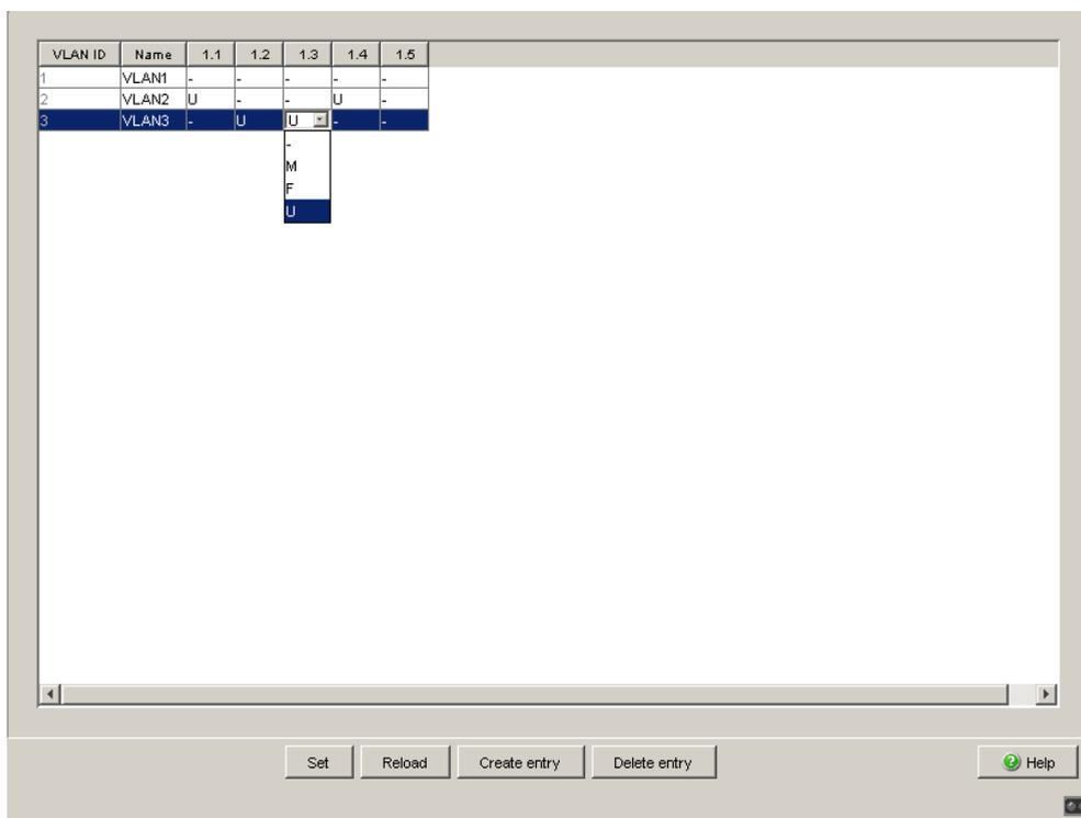
*Figure 45: Defining the VLAN membership of the ports.*
