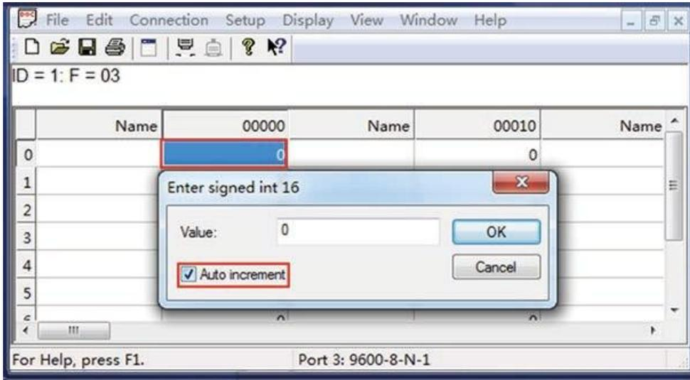
Figure 23 Modbus slave register value auto increment
