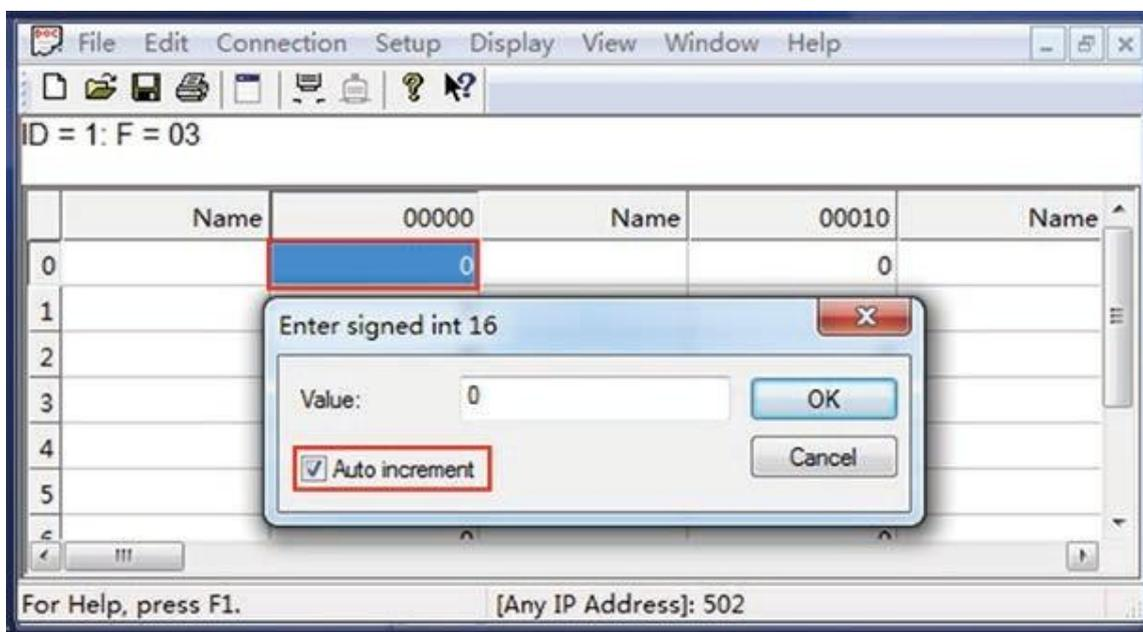
Figure 16 The value of Modbus slave register is automatically incremented
