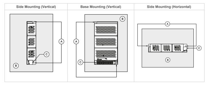
Fig. 2 Mounting Orientation
