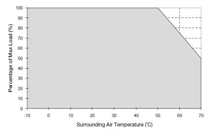
Fig. 1 De-rating for Vertical and Horizontal Mounting Orientation  $> 50^{\circ}\text{C}$  de-rate power by 2.5% /  $^{\circ}\text{C}$
