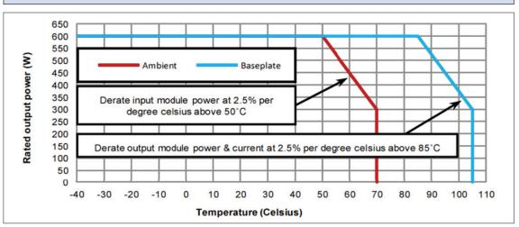
Apply appropriate derating to converter and modules for both ambient and baseplate temperatures
