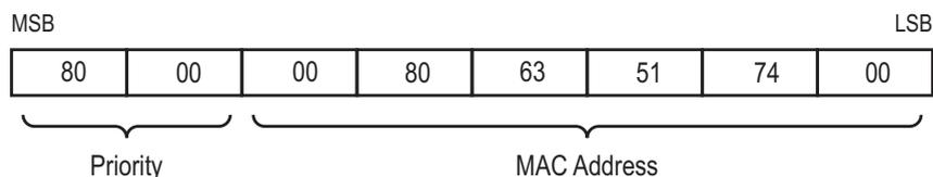
Figure 41: Bridge Identifier, Example (values in hexadecimal notation)
