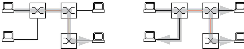
*Figure 2: MAC Data Transmission: Unicast Data Packet (left) and Broadcast Data Packet (right)*
