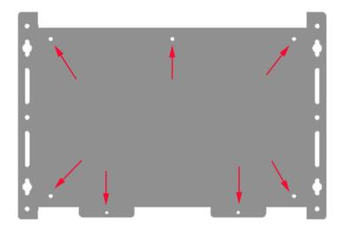
If you need to remove the motherboard, install or replace the 2<sup>nd</sup> memory module, move the jumper caps, or replace the lithium battery, you need to remove the 8 screws indicated below.
