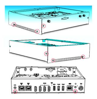
Below is a picture showing the device after removing the 8 screws just indicated.
