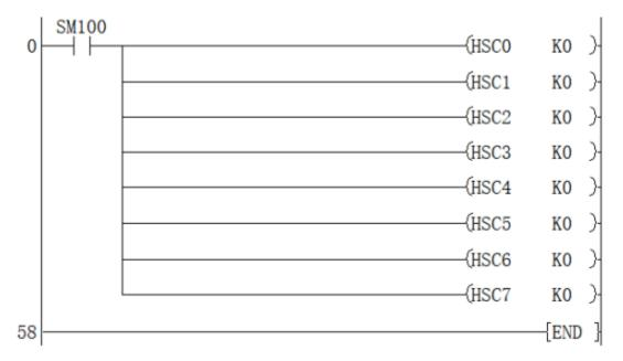
In the double word composed of special soft components SD403 and SD402, the current input pulse frequency of HSC0 can be monitored. Other channels also have corresponding registers, please refer to the description of special registers for details.
