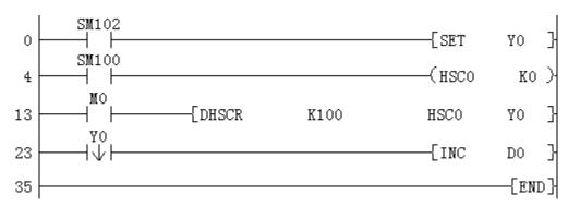
Use the OUT HSC instruction to turn on the high-speed counter while scanning MAIN.
