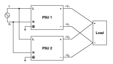
Fig. 4 Parallel Operation Connection Diagram
