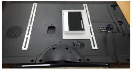
3. Install the TV mounting black bracket on the SI-22 silver-color mounting bracket.
