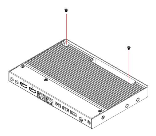
You can install SI-22 on plastic (LCD monitor), wood, drywall surface over studs, or a solid concrete or metal plane directly. Ensure the installer uses at least two M3 length 6mm screws to secure the system on the wall. *Four M3 length 6mm* screws are recommended to secure the system onto the wall.
