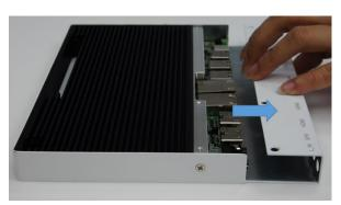
2. Push the mSATA module into the slot. Screw two screws to secure the module in the slot.
