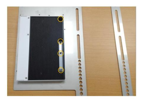
2. Please install mounting bracket to the mounting hole of display which you use. Depending on the application, there are different orienations, as shown below.
