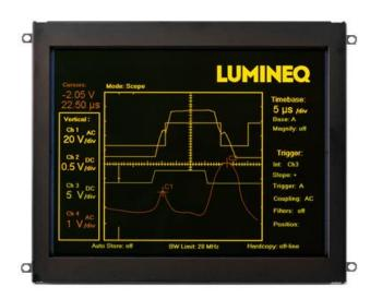
The EL640.480-AA1 is a multi-color VGA display for use in extreme operating conditions.
