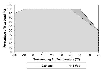
**Fig. 1 De-rating for Vertical Mounting Orientation** -10°C to -20°C de-rate power by 1% / °C > 40°C de-rate power by 1.67% / °C @ 115 Vac
