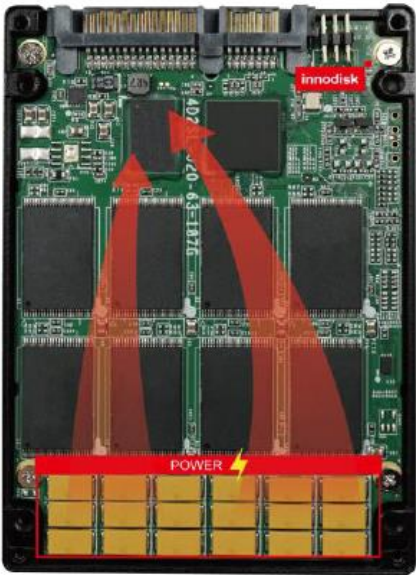
Figure 3: Diagram of 2.5" SATA SSD with iCell
