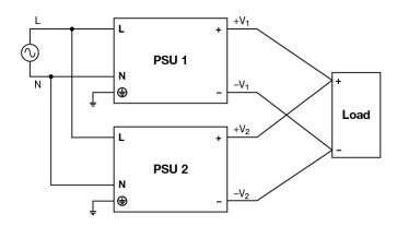
Fig. 4 Parallel Operation Connection Diagram
