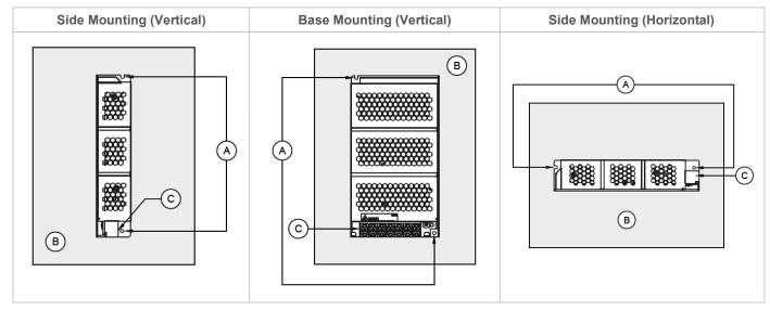
Fig. 2 Mounting Orientation
