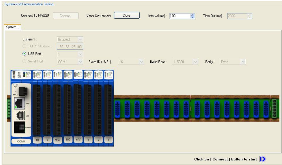
Figure 8: MAQ20-940 ReDAQ Shape for MAQ ® 20 Main Configuration Screen
