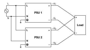
Fig. 4 Parallel Operation Connection Diagram
