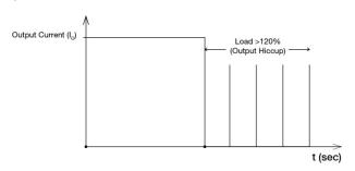
It is not recommended to prolong the duration of  $I_0$  when it is <120% but >100%, since it may cause damage to the PSU.
