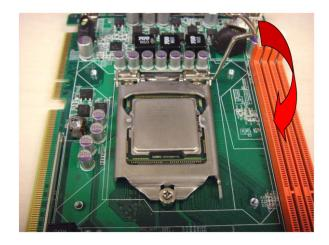
5. The finished processor installation.
