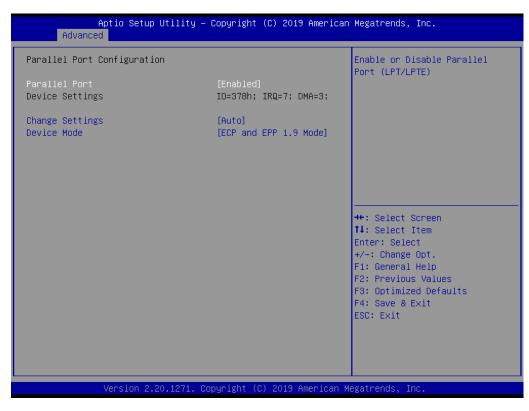
Figure 3.32 Parallel Port Configuration
