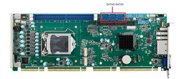
The PCE-7132/5132/5032 features high performance serial ATA interface (5\*600MB/ s) which eases cabling to hard drivers or CD/DVD drivers with long cables. These five on-board SATA ports can be configured as RAID 0, 1, 10, or 5 (PCE-5132 do not support RAID). Please see the detailed BIOS setting instructions for this in Chapter 3.
