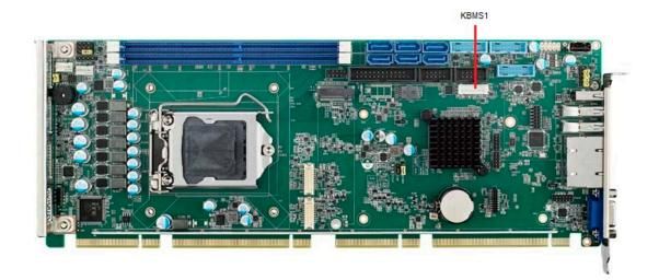
The on-board KBMS1 pin header provides connection to the front panel PS/2 keyboard and mouse connector of the chassis.
