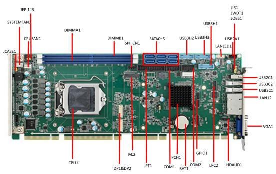
Figure 1.1 Jumper and Connector Locations
