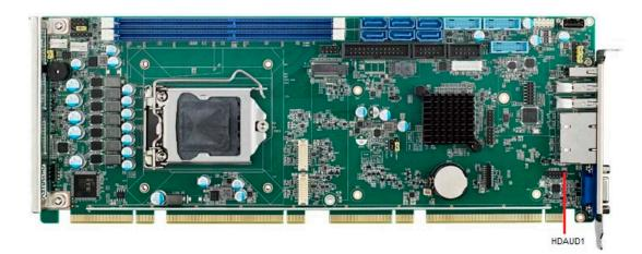
This HDAUD1 pin header is the connection interface to Advantech's high definition audio module.
