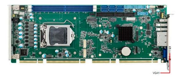
This CPU card has VGA outputs that can drive conventional CRT displays. VGA1 is a standard 15-pin D-SUB connector commonly used for VGA.
