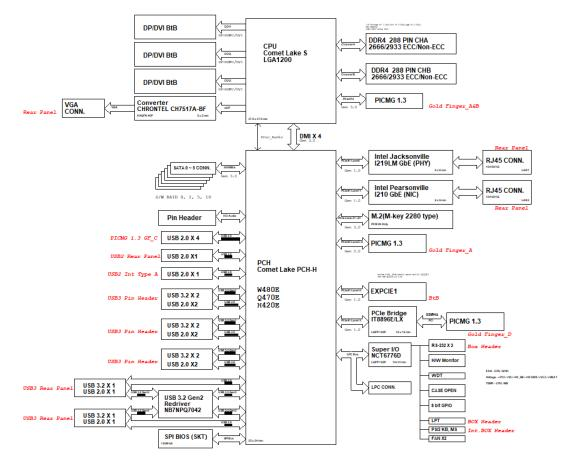
Figure 1.2 PCE-7132/5132/5032 Block Diagram
