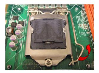
Remove the socket protection cap. 2.
