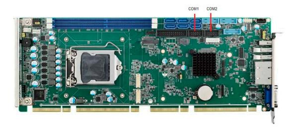
These SBCs offer two serial ports. These ports can connect to serial devices, such as a mouse or a printer, or to a communications network.
