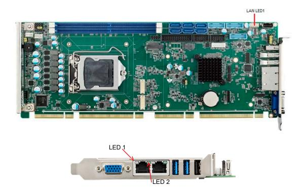
The SBC is equipped with one or two high-performance 1000 Mbps Ethernet LANs. They are supported by all major network operating systems. The RJ-45 jacks on the rear plate provide convenient connectivity.
