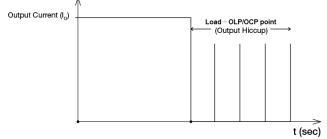
It is not recommended to prolong the duration of  $\rm I_{O}$  when it is less than OLP/OCP point, but greater than 100%, since it may cause damage to the PSU.
