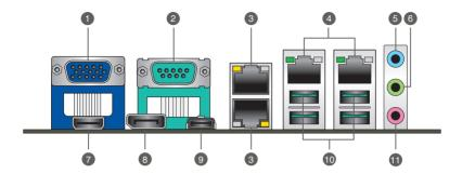
Video Graphics Adapter (VGA) port. This 15-pin port is for a VGA monitor or other VGA-compatible devices.
