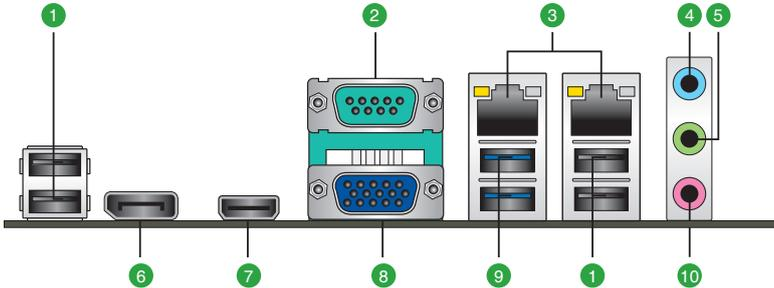
1. **USB 2.0 ports.** These 4-pin Universal Serial Bus (USB) ports are for USB 2.0 devices.
