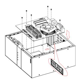
Figure 2.2 Installing a motherboard
