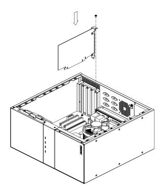
Figure 2.3 Installing an add-on card
