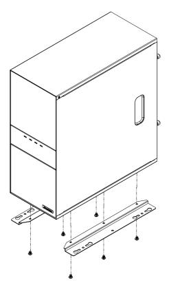
Figure 2.6 Installing wallmount brackets
