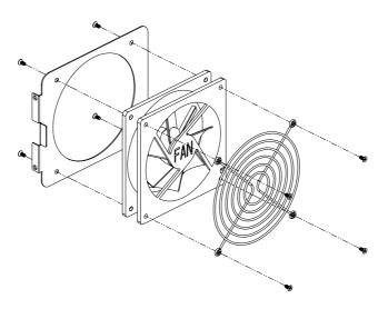
Figure 3.5 Replacing the cooling fan from fan bracket
