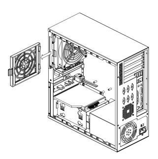
Figure 3.6 Replacing the filters
