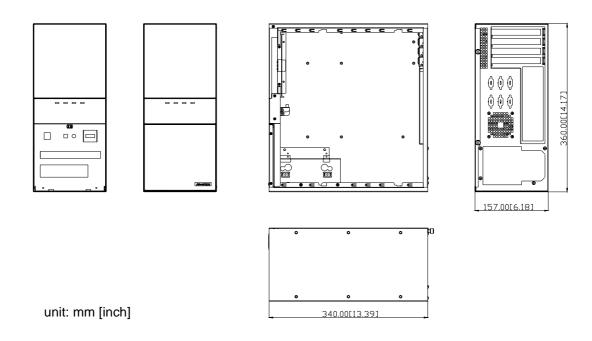
Figure 1.1 Dimension diagram
