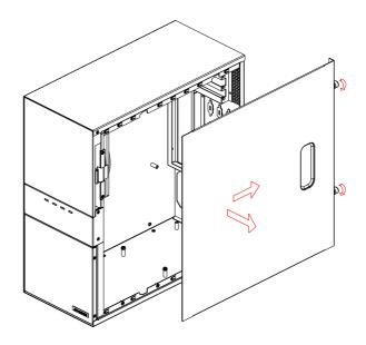
Figure 2.1 Removing the side cover
