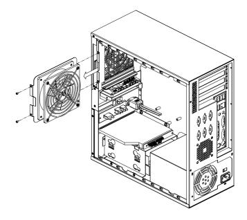
Figure 3.4 Replacing the cooling fan
