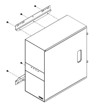
Figure 2.7 Installing wallmount brackets
