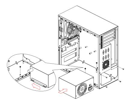
Figure 3.7 Replacing the single power supply
