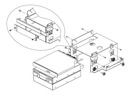
Figure 2.4 Installing 3.5" HDD disk drive, FDD and slim ODD
