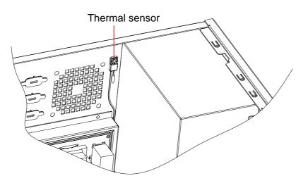
Figure 4.2 Thermal sensor location
