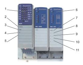
Figure 13: Labels for basic modules and media modules
