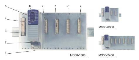
Figure 5: Overview of interfaces, display and operating elements on the MS30
