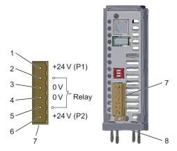
Figure 17: Pin assignment of the 6-pin terminal block
