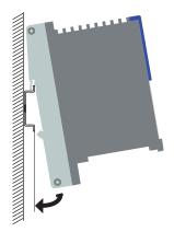
The lower panel of the device casing is grounded via the DIN rail and optionally by means of the separate ground screw. See figure 2 on page 25.
