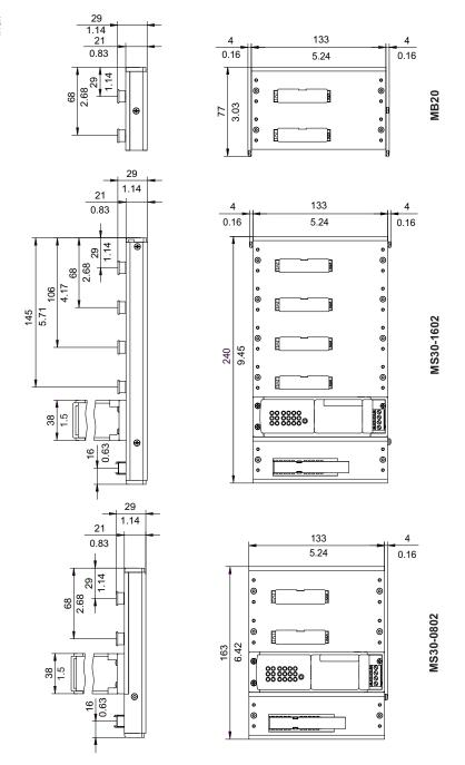
Figure 21: Dimensions of base module MS30 variants and extender module
