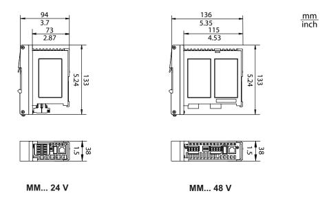
Figure 22: Dimensions of media modules
