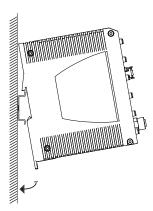
To mount the device onto a horizontally mounted 35 mm DIN rail according to DIN EN 60715, proceed as follows:
