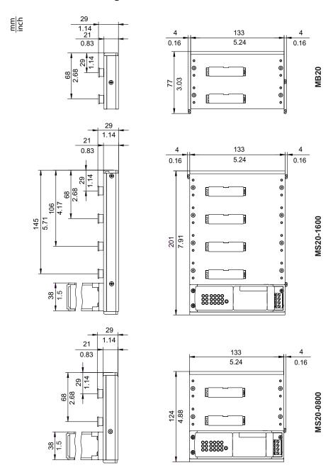
Figure 20: Dimensions of base module MS20 variants and extender module
