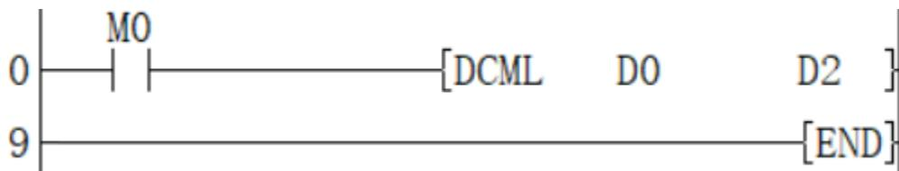
When M0 is set, the value of (D1, D0) is reversed and transferred to the value of (D3, D2).
