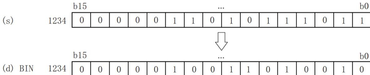
GRY→BIN Mathematical Algorithm: Starting from the second bit from the left, XOR each bit with the decoded value of the left bit as the decoded value of the bit (the leftmost bit remains unchanged).
