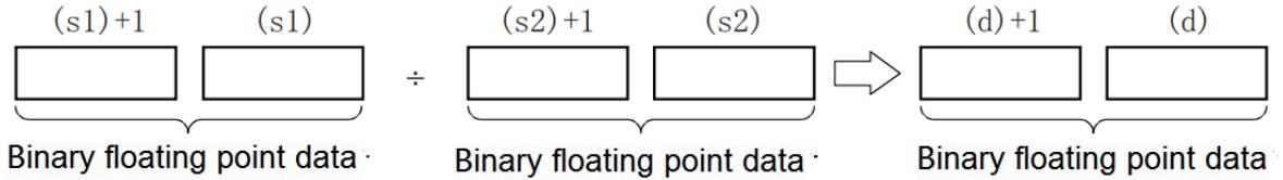
When constants (K, H) to (s1), (s2) are specified, the value is automatically converted to a binary floating point data.
