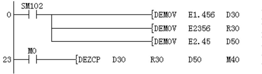
Since 2.45 is greater than 1.456 and 2.45 is less than 2356, M41 is set to ON
