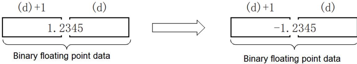
Used when inverting positive and negative signs.
