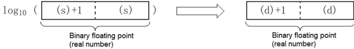
The value specified in (s) can only be set to a positive number. (Cannot perform operations with negative numbers.)
