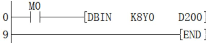
When M0 is set, the BCD value of K8Y0 is converted into BIN and stored in D200.
