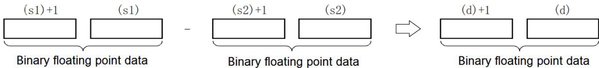
When constants (K, H) to (s1), (s2) are specified, the value is automatically converted to a binary floating point data.
