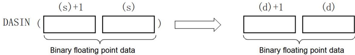
The SIN<sup>-1</sup> value specified in (s) can be set within the range of -1.0 to 1.0.
