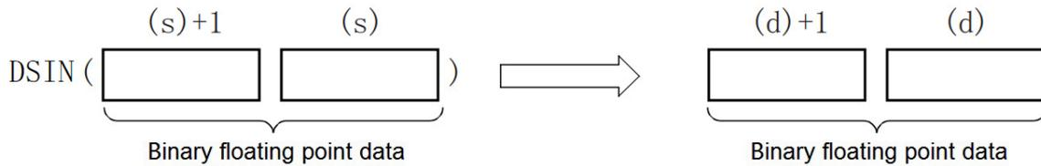
For the angle specified in (s), set it in radians ( $\text{angle} \times \pi \div 180$ ).
