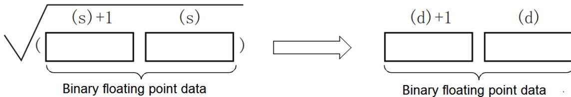
The value specified in (s) can only be set to a positive number. (Cannot perform operations with negative numbers.)
