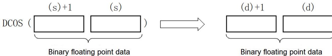
For the angle specified in (s), set it in radians ( $\text{angle} \times \pi \div 180$ ).
