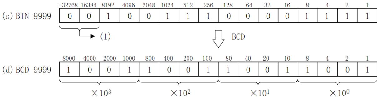
The data specified in (s) can be converted in the range of K0 to K9999 by BCD (decimal number).
