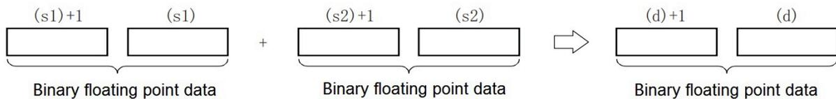
When constants (K, H) to (s1), (s2) are specified, the value is automatically converted to a binary floating point data.
