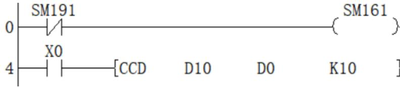
Regarding D10 as the initial 10-point data, the addition data and horizontal parity data of the high and low 8-bit data are stored in the Devices of D0 and D0+1.
