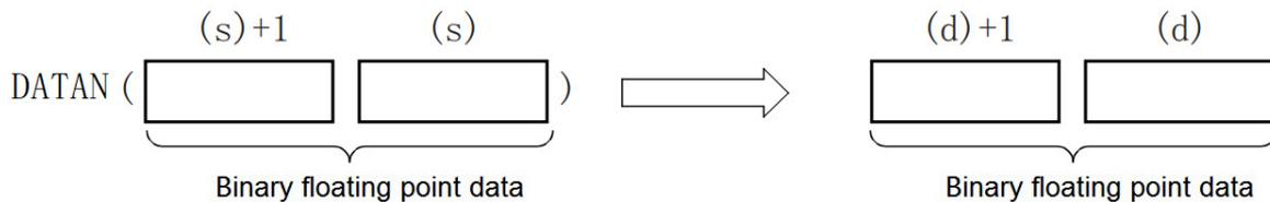
The angle (calculation result) stored in (d) is stored in the unit of radians ( $-\pi/2$ ) to ( $\pi/2$ ).
