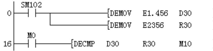
Since the floating point number in R30 is greater than the floating point number in D30, M12 turns ON.
