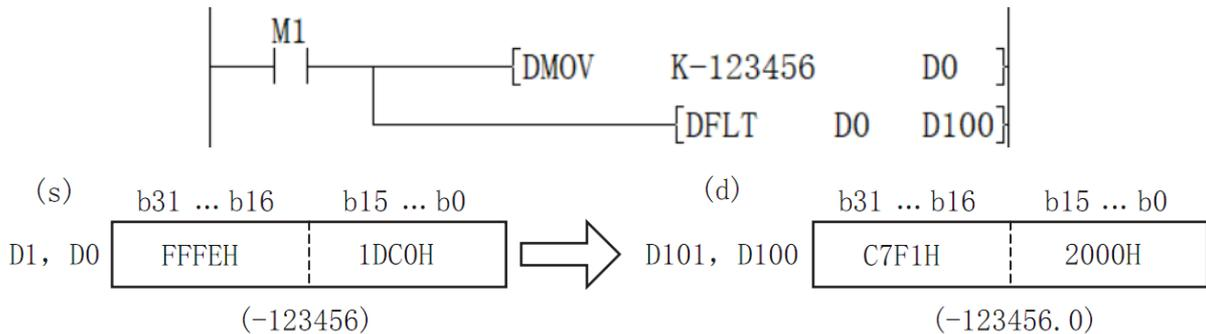
**#Note:** In each binary floating-point number (real number) operation instruction, the specified K and H values are automatically converted into a binary floating-point number (real number), so there is no need to use the DFLT instruction for conversion. The inverse conversion instruction of this instruction is INT (convert a binary floating point value into a BIN integer).
