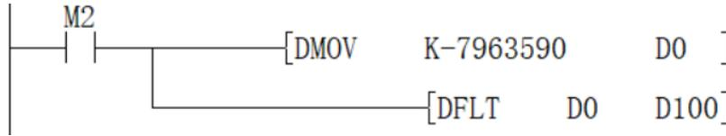
When M2=ON, convert the BIN 32-bit integer -7963590 in [D1, D0] into a single-precision floating point number -7963590.0 and store it in the [D101, D100] device.
