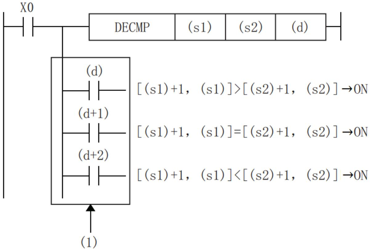
(1): Even if the command input is turned OFF and the DECMP command is not executed, (d) to (d)+2 will keep the state before X0 is turned OFF.
