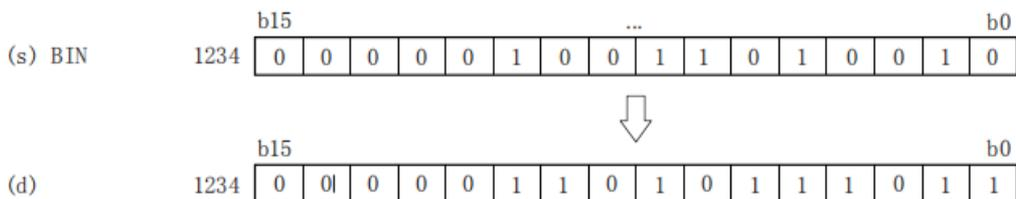
BIN→GRY Mathematical Algorithm: Starting from the rightmost bit, XOR each bit with the left bit as the value corresponding to the GRY bit, and the leftmost bit remains unchanged (equivalent to 0 on the left) .
