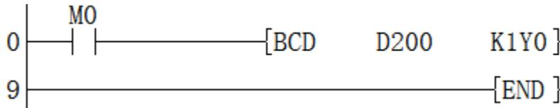
When M0 is set, the BIN value of D200 is converted into BCD and stored in K1Y0.
