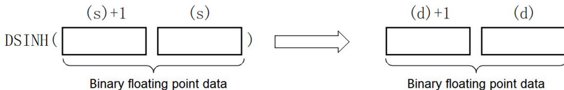
The instruction is to take the SINH value from a binary floating point number. The calculation formula is  $\sinh \text{ value} = (e^s - e^{-s})/2$ .
