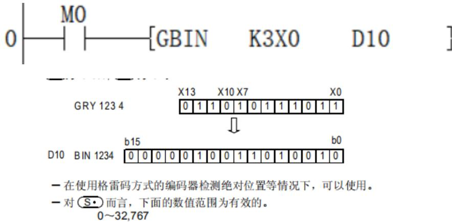
It could be used when the encoder of Gray code method is used to detect the absolute position.
