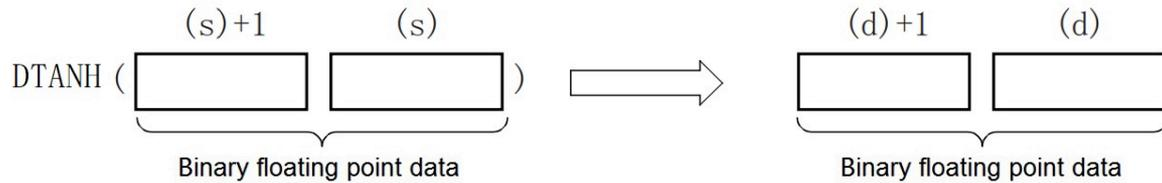
The instruction is to take the TANH value of a binary floating point number. The calculation formula is  $\tanh \text{ value} = (e^s - e^{-s}) / (e^s + e^{-s})$ .
