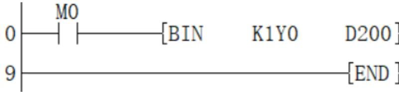
When M0 is set, the BCD value of K1Y0 is converted into BIN and stored in D200.
