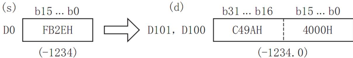
**#Note:** In each binary floating point number (real number) operation instruction, the specified K and H values will be automatically converted into a binary floating point number (real number), so there is no need to use the FLT instruction for conversion.
