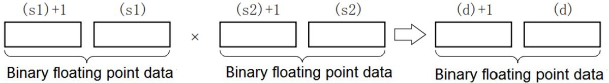
When constants (K, H) to (s1), (s2) are specified, the value is automatically converted to a binary floating point data.
