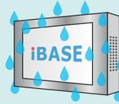
Protected against vertically falling drops of water. Limited ingress permitted.
