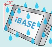
Protected against vertically falling drops of water with enclosure tilted up to 15 degrees from the vertical. Limited ingress permitted.
