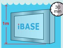
Protection against the effects of immersion in water between 15 cm and 1 m for 30 minutes.
