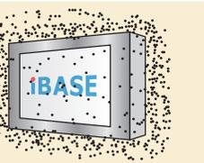
Dust protected. Limited ingress of dust permitted. Will not interfere with operation of the equipment. Two to eight hours.
