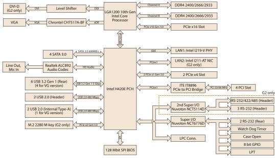
Figure 1.3 Block Diagram
