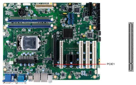
The AIMB-707 provides a PCIe x16 slot for users to install an add-on peripheral card for extension requirements.
