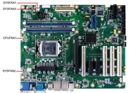
If a fan is used, this connector supports cooling fans that draw up to 500 mA (6 W).
