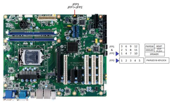
There are several external switches and LEDs to monitor and control the AIMB-707.
