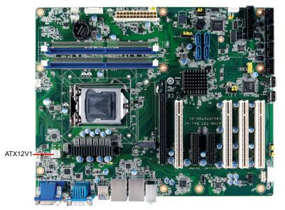
To ensure that enough power is supplied to the CPU, one auxiliary 8-pin power connector is available on the AIMB-707. ATX12V1 must be used to provide sufficient 12 V power to ensure the stable operation of the system.
