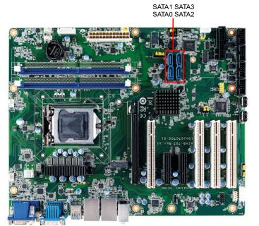
AIMB-707 features four high performance serial ATA 3.0 interfaces (up to 600 MB/s) with long, thin, easy-to-run SATA cables.
