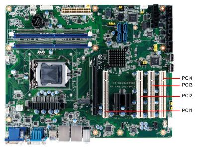
The AIMB-707 provides four 32-bit / 33 MHz PCI slots.
