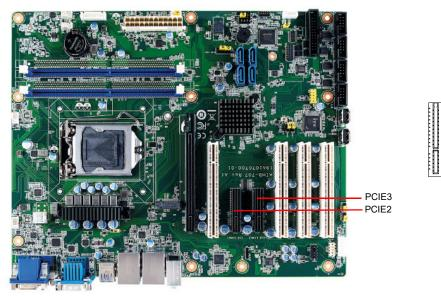
The AIMB-707 offers two PCIe x4 slots for users to install add-on cards for extension requirements. PCIE2 and PCIE3 are PCIe x1 link.
