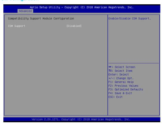
Figure 3.28 CSM Configuration
