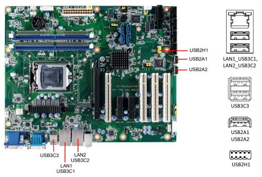
The AIMB-707 is equipped with up to two high-performance 1000 Mbps Ethernet LANs. They are supported by all major network operating systems. The RJ-45 jacks on the rear plate provide convenient 1000Base-T operation. VG sku provides single GbE LAN only.
