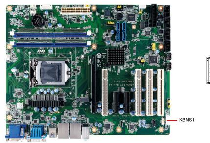
A 6-pin header (KBMS1) on the motherboard is for an optional PS/2 keyboard/mouse cable. This gives system integrators greater flexibility in designing their systems.
