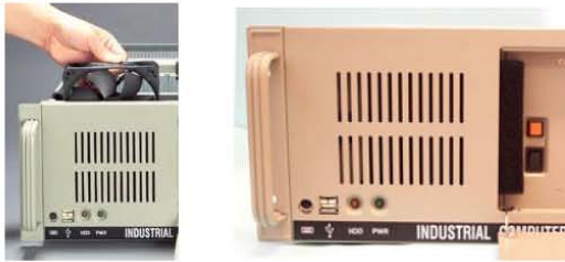
Figure 2-3 Cooling fan & filter
