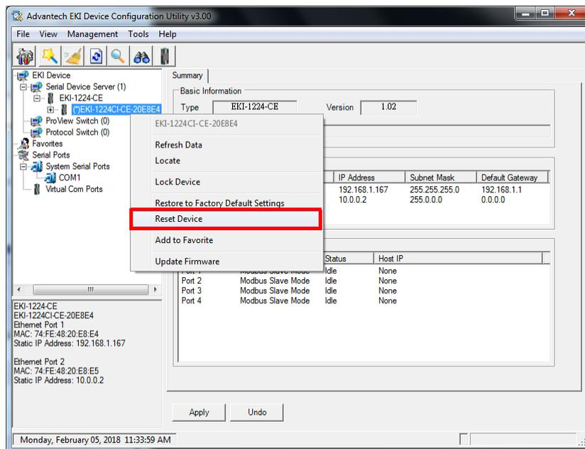
**Figure 3.15 Reset Device**
