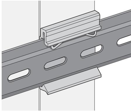
**Figure 2.14 Correctly Installed DIN Rail Kit**
