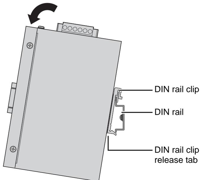
Figure 2.13 Installing the DIN-Rail Mounting Kit
