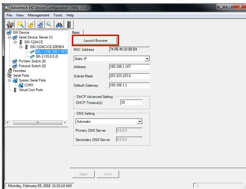
**Figure 4.1 Accessing the Web Page via Configuration Utility**
