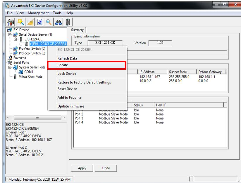
**Figure 3.16 Locate the Serial Device Server**
