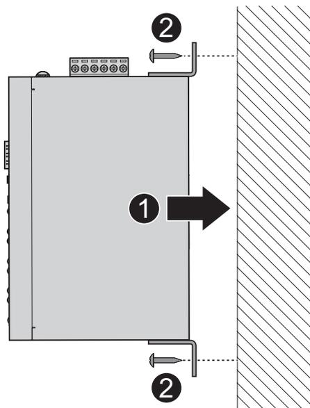
**Figure 2.18 Wall Mount Installation**
