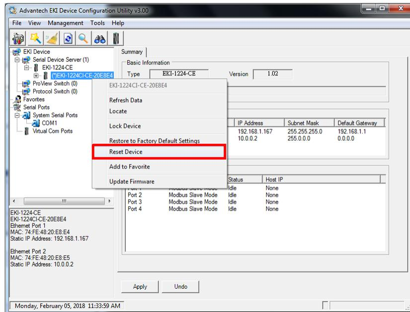
**Figure 3.22 Reset Device**
