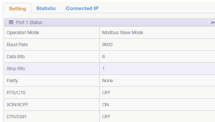
The screenshot shows a web interface with three tabs: 'Setting' (selected), 'Statistic', and 'Connected IP'. Below the tabs is a table titled 'Port 1 Status'. The table has two columns: the parameter name and its current value.
