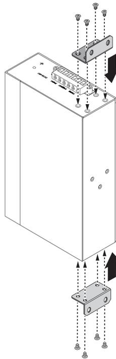
**Figure 2.16 Installing Wall Mount Plates**
