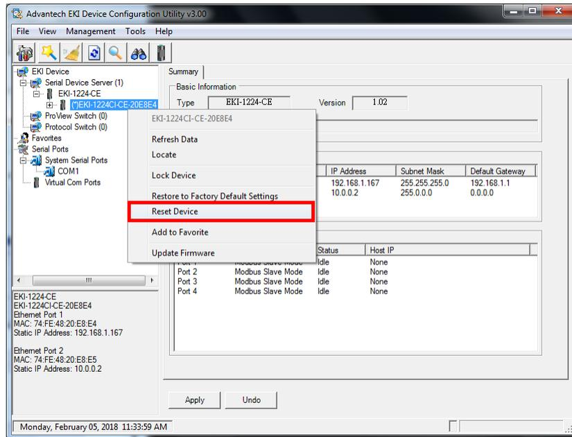
**Figure 3.19 Reset Device**
