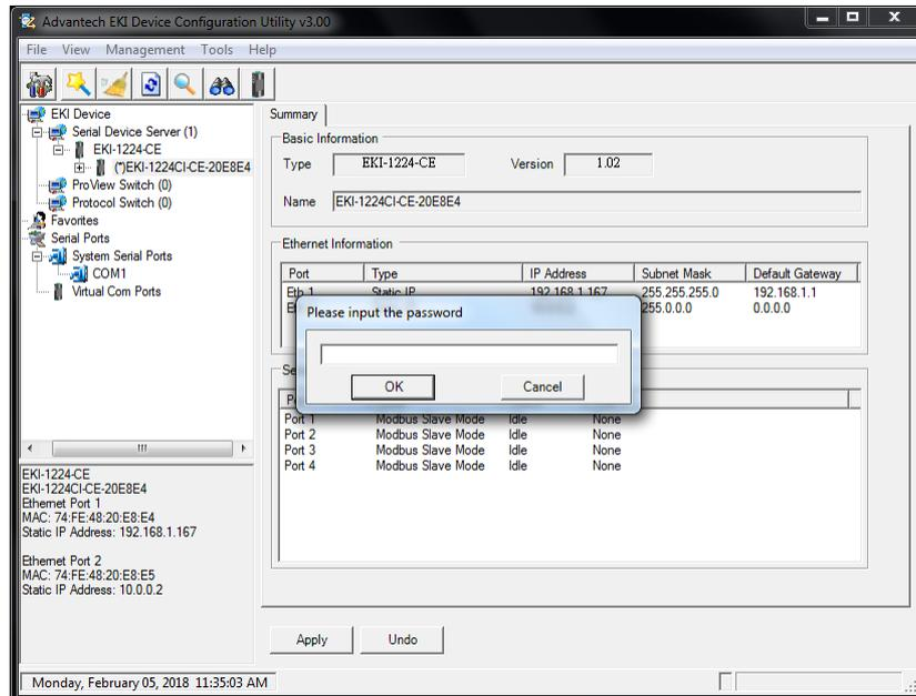
**Figure 3.20 Unlock the Serial Device Server**
