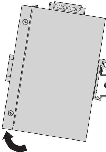
**Figure 2.15 Removing the DIN-Rail**
