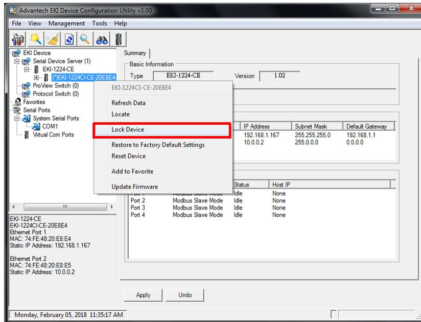
Figure 3.17 Lock the Serial Device Server
