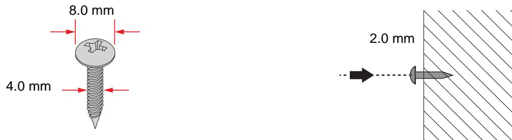
**Figure 2.17 Securing Wall Mounting Screws**
