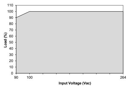
Fig. 2 De-rating for AC Input Voltage < 100 Vac de-rate power by 1 % / Vac
