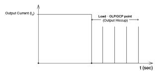
It is not recommended to prolong the duration of  $I_{\rm O}$  when it is less than OLP/OCP point, but greater than 100%, since it may cause damage to the PSU.
