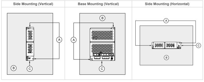
Fig. 2 Mounting Orientation
