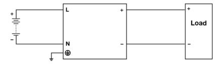
Fig. 3 DC Input Operation Connection Diagram
