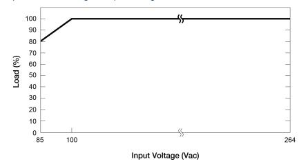
No output power de-rating for the input voltage from 100 Vac to 264 Vac
