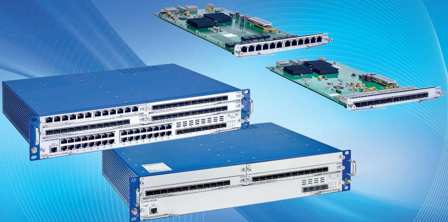
The Hirschmann DRAGON MACH4x00 series offers an innovative, technically-advanced architecture that delivers superior bandwidth for connecting OT and IT networks.
