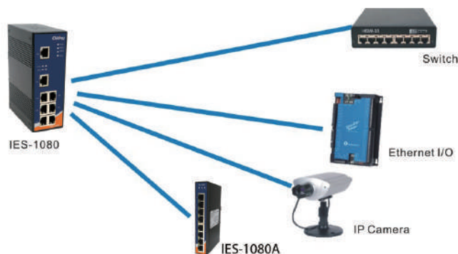
Connections of Ethernet devices
