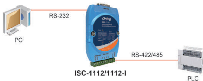
Connections of Serial Media Converter
