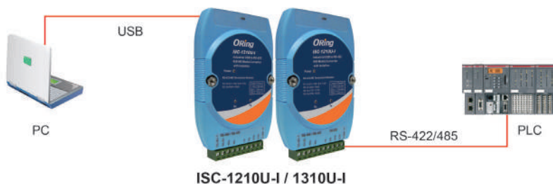
Connections of USB to Serial Media Converter
