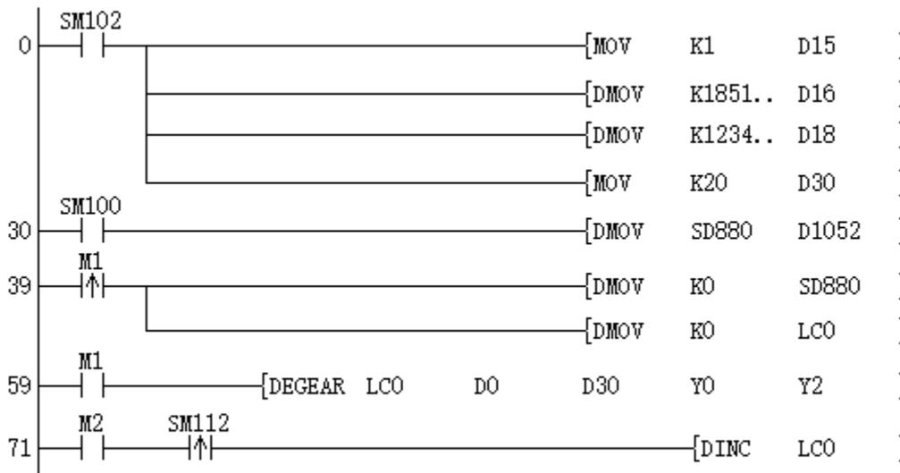
Set the 32-bit gear ratio: 18518517: 12345678, set the 15 address of the data buffer to 1, and enable the 32-bit gear ratio function.
