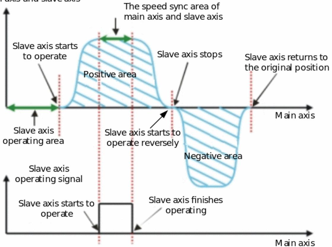
The stroke of the flying saw is divided into two parts: the following part and the returning part. The two moving distances must be the same. From the speed stroke point of view, that is, positive area = negative area.
