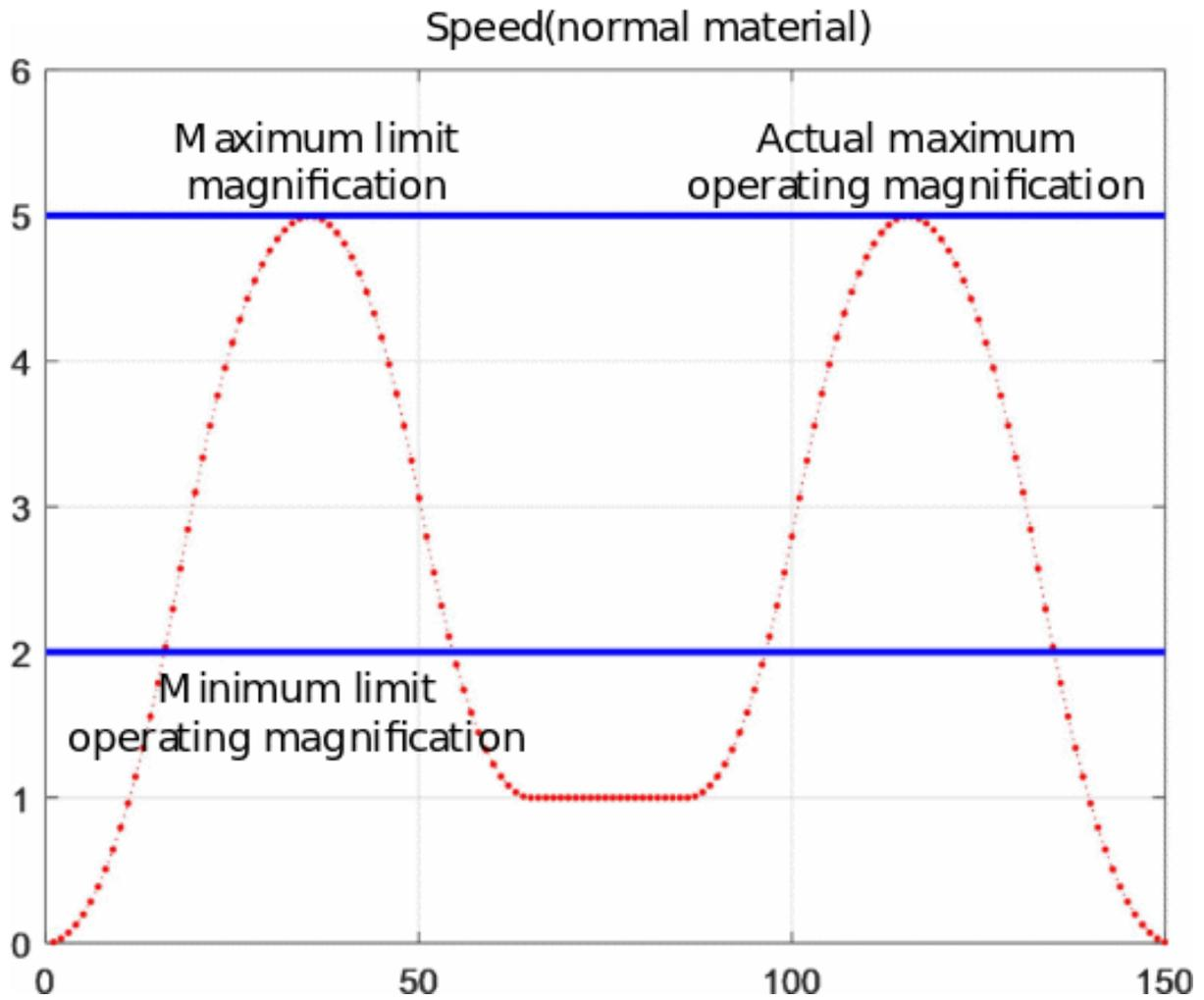
③The shortest length of material (Lm3): the actual maximum operating magnification = the minimum limit operating magnification, the adjustment area is acceleration + deceleration + dwell process.
