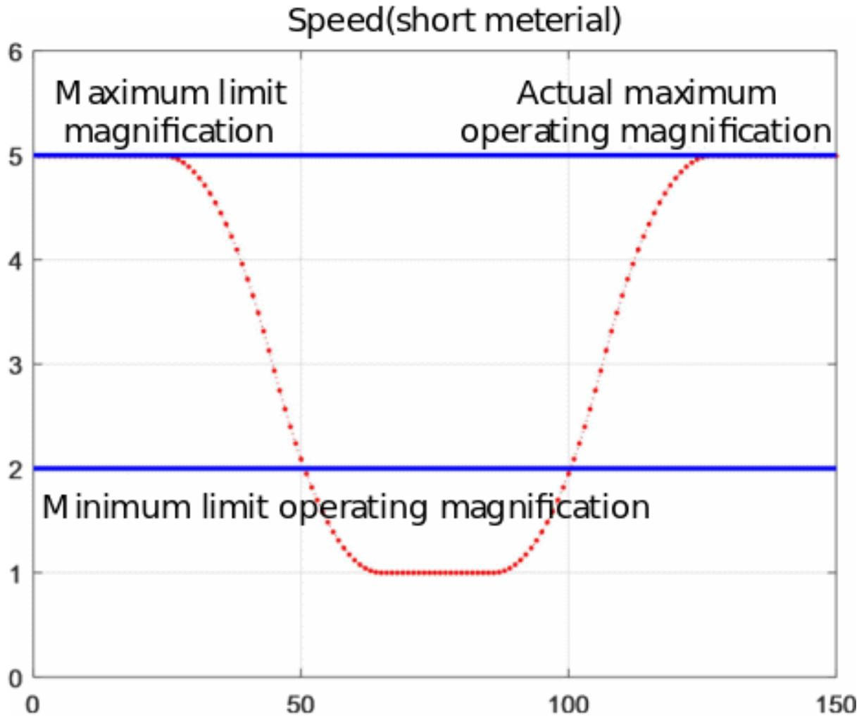
②The shortest normal material (Lm2): the actual maximum operating magnification = the maximum limit magnification, the adjustment area is the acceleration + deceleration process.
