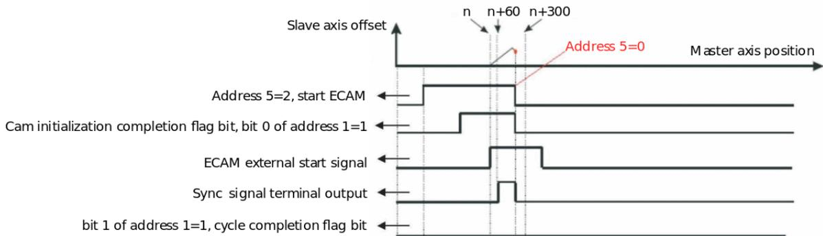
2. When the aperiodic ECAM is running, address 4-BIT1=1 (stop after the current cycle is completed), the aperiodic ECAM will continue to run through the table and then the slave axis will stop operating, as shown in the figure below.
