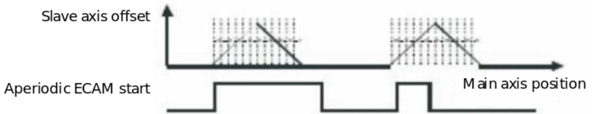
**(8) Address 15-16—Electronic cam start delay pulse setting**
