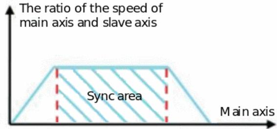
Cutting length > 2 times the circumference of the cutter: When the cutting length is greater than 2 times the knife circumference (this is also the most common situation), in a cycle, after the cutting of the knife edge in the synchronization zone is completed, it decelerates to a stop, waits for a certain length to pass, and then starts the next cutting.
