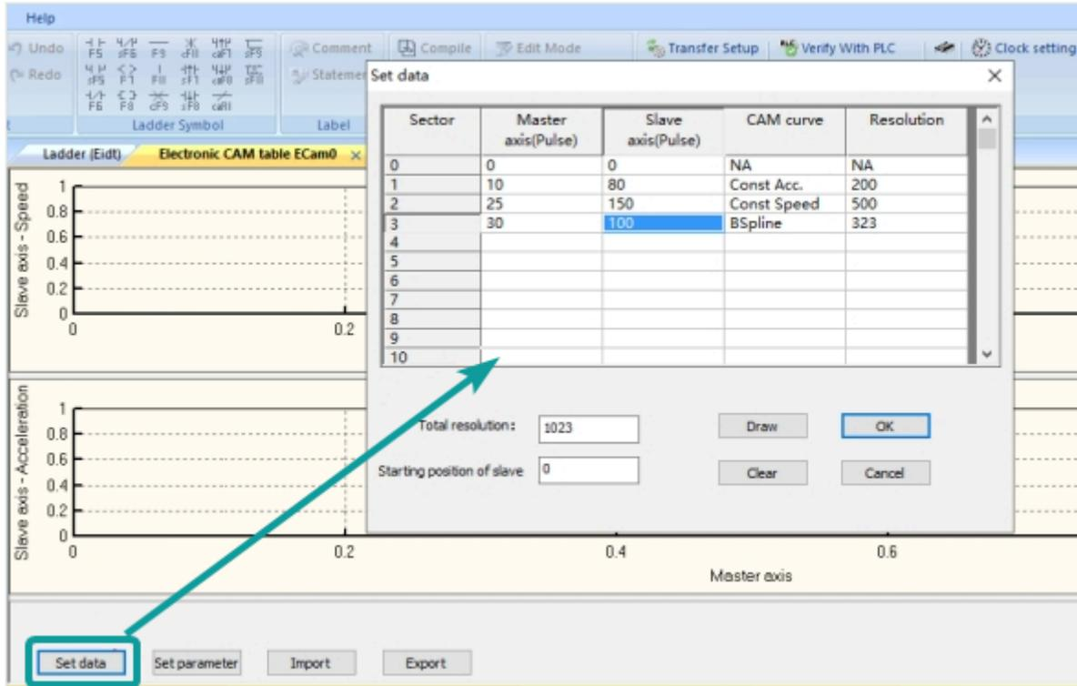
[Data Setting] The window is composed of sections, each section provides the user to set a section of cam curve, and then the entire section composes the cam curve. Each section is composed of master axis, slave axis, CAM curve and resolution, as explained below:
