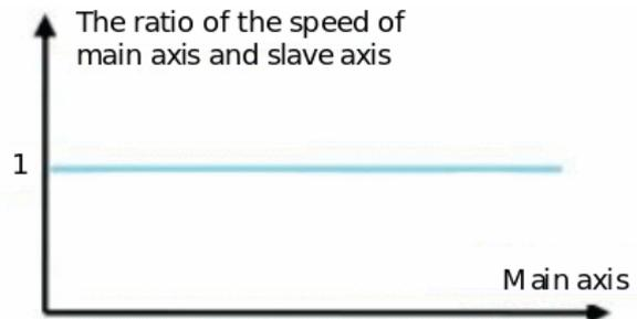
1 times cutter circumference < cutting length < 2 times cutter circumference: After the cutting action in the synchronization zone is completed, the cutting axis decelerates, then speed up to synchronize the next cutting, as shown in the figure.
