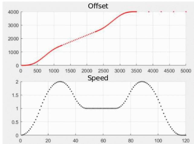
② Synchronous magnification = minimum limit operation magnification < maximum limit magnification
