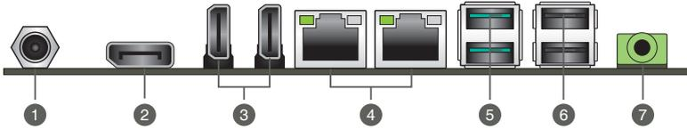
1. **DC Power connector.** Insert the power adapter into this port.
